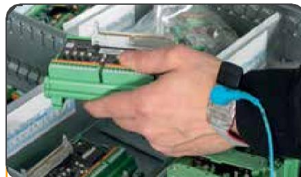
ESD Protection System
